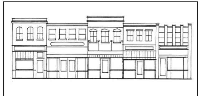
Figure 5.10. Minor changes in roof heights, materials and details can break up long building facades.
