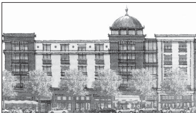
Figure 5.6. To avoid a large undifferentiated facade, provide articulation through changes in the planes, materials and colors.
