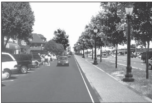
Figure 3.9. Service roads can provide connections between adjacent commercial uses, limiting the need to travel along arterial highways.
