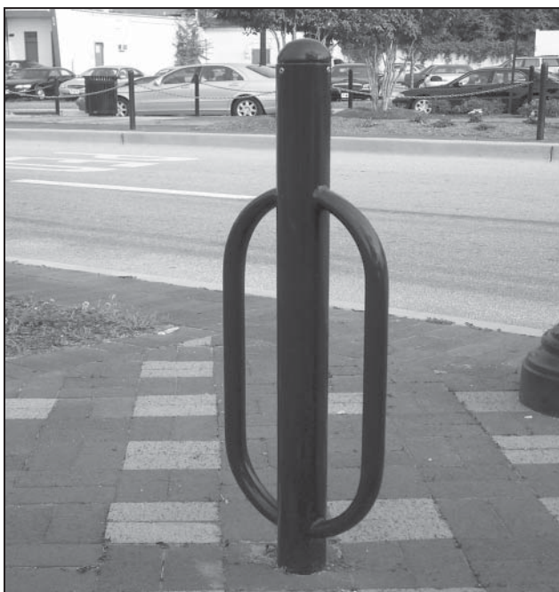
Figure 3.20. The recommended bollard for the Route 1 corridor is Bollard 35, BKR permanent mount, manufactured by Victor Stanley, Inc., or equal by another manufacturer. The bollard can also serve as a bicycle storage area.
